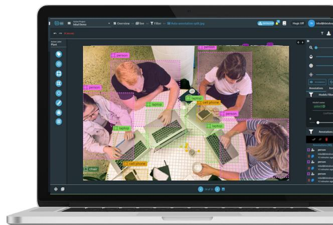
**Fig-2:** Using built-in object detection models to pre-label the data. Model results are visualized on top of the image and can be filtered based on model confidence scores, allowing human labelers to quickly validate and edit model outputs.
